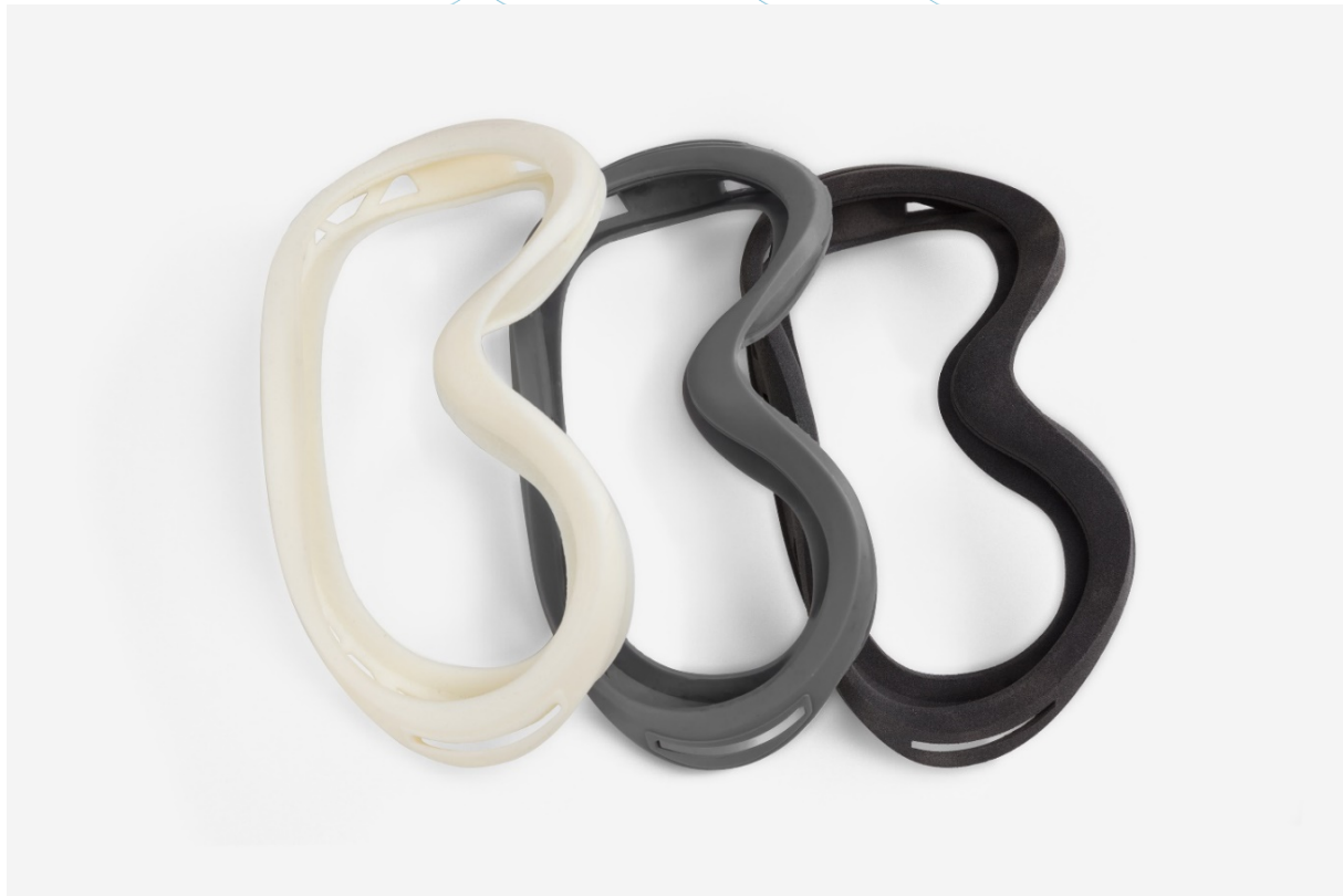
Figure 5: Prototypes of a ski goggles' frame printed with FDM, SLA and SLS technology (from left to right). [9]
