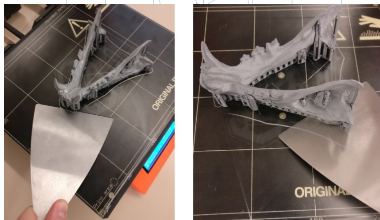
Figure 65: Piece extraction process. [90]
