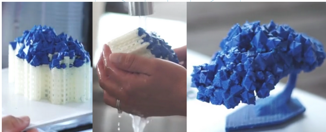
Figure 37: Bath for removing the support structures. [51]
