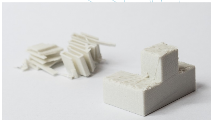
Figure 49: FDM printed puzzle piece with support removed showing surface roughness. [73]
