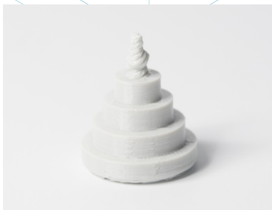
Figure 53: Print of vertical pins with decreasing diameter (from 25 to 5mm) illustrating the upper diameter of the print becoming too small to print accurately. [77]
