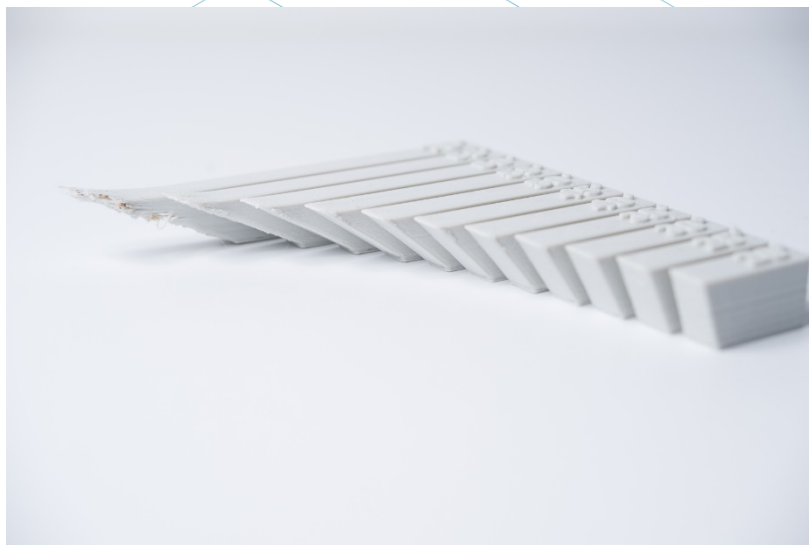
Figure 51: The effect of increasing overhang angle (in increments of 5 degrees) on print quality. Max. angle shown is 70 degrees. [75]
