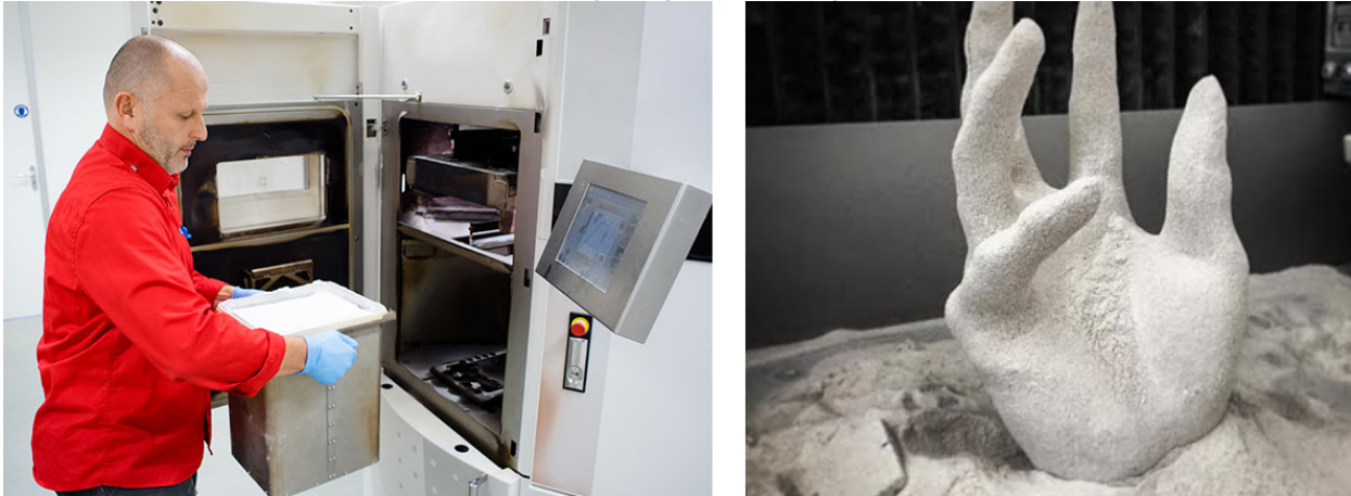
Figure 34: SLS extraction process. [48]
